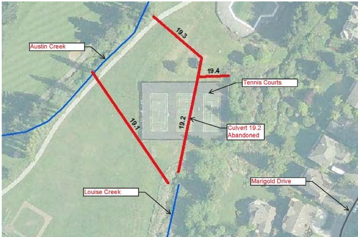
Aerial photo showing culvert path through adjacent field.
