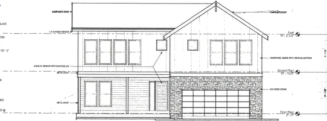
① FRONT ELEVATION 1/4" = 1'-0"
