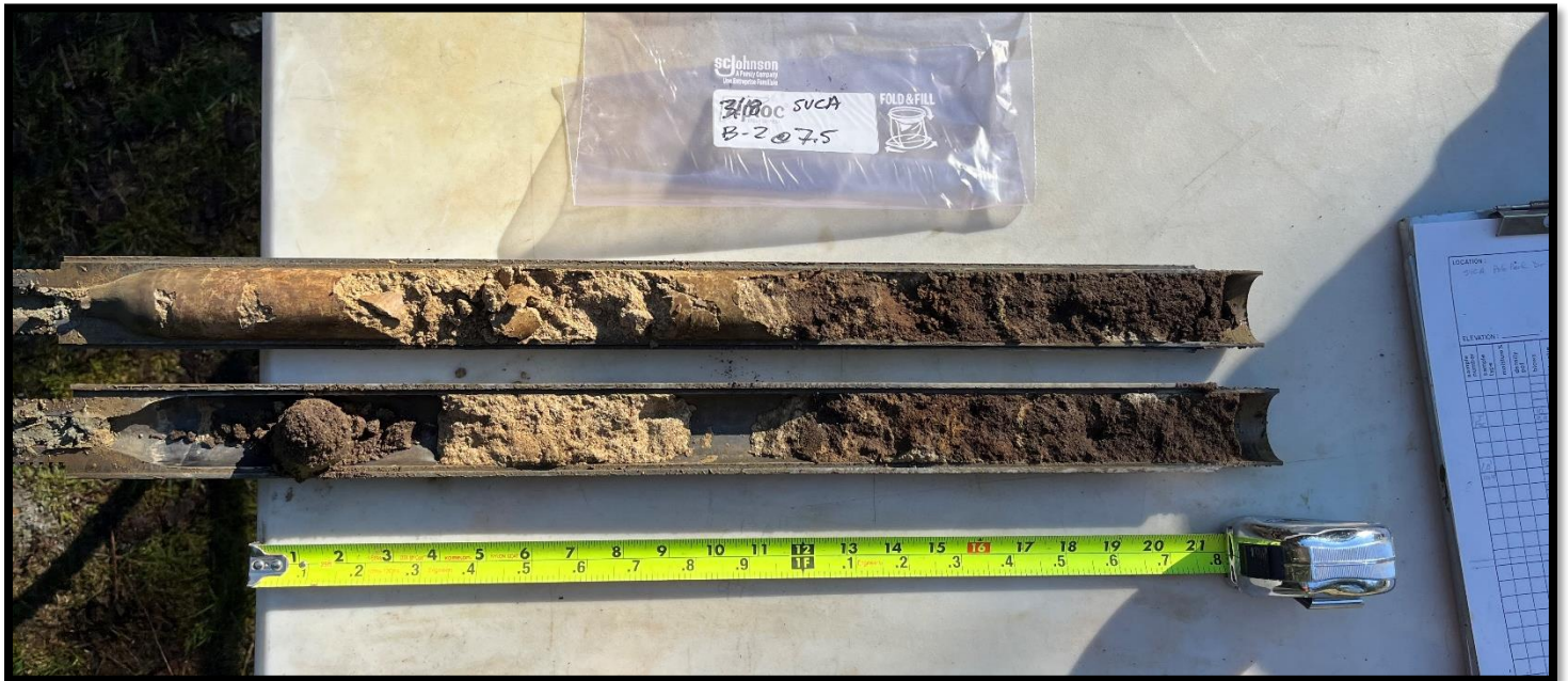
Photo 5: Borehole B-2 at 7.5 feet BPG showing weathered Chuckanut Formation sandstone bedrock on March 18, 2024.
