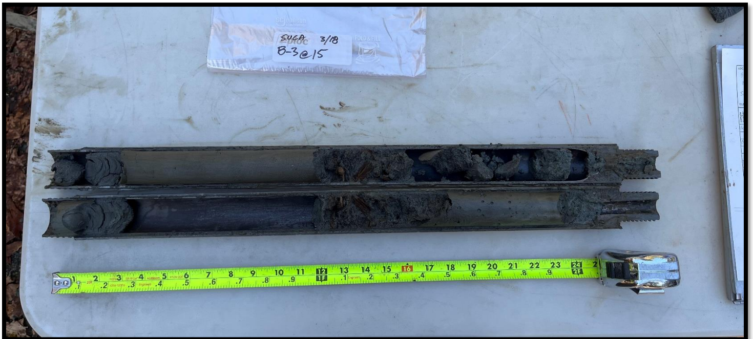
Photo 6: Borehole B-3 at 15 feet BPG showing lacustrine (lake) deposits with notable organic content on March 18, 2024.
